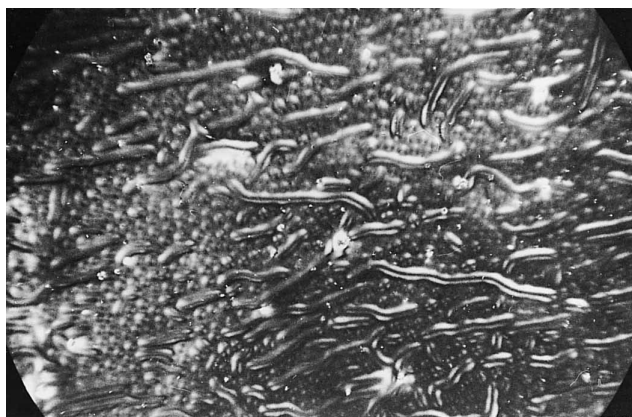
Figure 4. Cross-like domains and \pi -walls in MBBA nematic layer with a thickness of 42\ \mu\text{m} , crossed polarizers, an applied d.c. voltage of 4 V, magnification 6 \times 10 , the long side of the photo corresponds to 1350\ \mu\text{m} .
