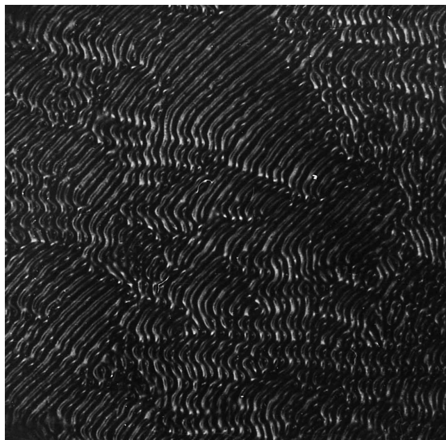
Figure 14. Undulations of the domains shown in figure 13 (a) under a d.c. voltage of 7 V.
